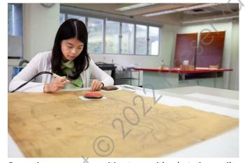
Removing pressure sensitive tape with a hot air pencil
